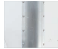
.125" Extruded-aluminum Radius Vertical Front Corners provide superior strength at the front of the body minimizing damage
