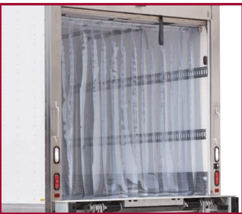
POPULAR OPTION Prevent heated air from entering the truck body while the door is open with a strip curtain
