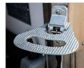
Refrigeration Unit Access Steps (4)
