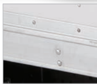
14-gauge Galvannealed Steel Lower Perimeter enhances impact resistance and durability behind the rub rail
