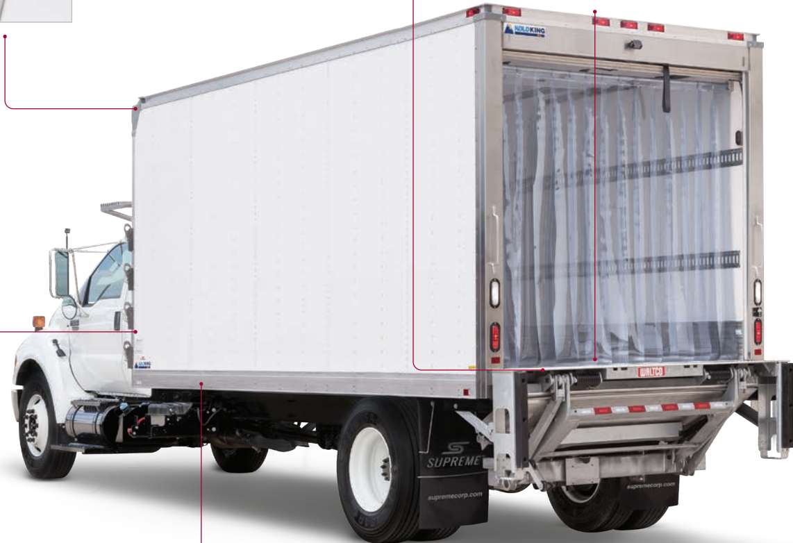
14-gauge Galvannealed Steel Lower Perimeter enhances impact resistance and durability behind the rub rail
