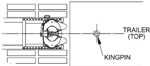
Inflate tractor air suspension and back up **close** to the trailer centering the kingpin with the throat of the fifth wheel and **STOP!**
