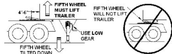
Adjust trailer height so that the fifth wheel will lift the trailer.
