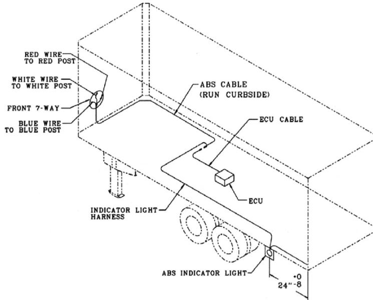
**ABS Electrical System Diagram**
