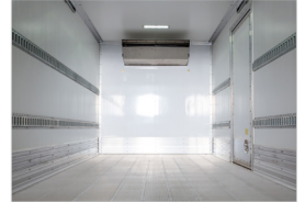
Anti-microbial composite interior liner
